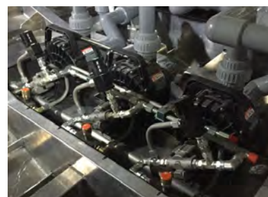
RSE2 2" hydraulic drive pumps installed on a fishing vessel
