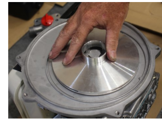
Mech seal installed in impeller
