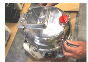
Tighten opposite bolts to apply even pressure
