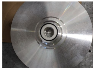
Mech seal installed in impeller
