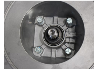
Counterface installed on engine shaft
