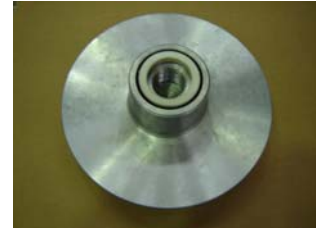
Transfer mech seal to new impeller
