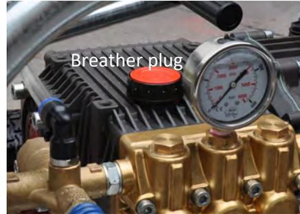
**WARNING:** Before operation ensure top mounted travel plug is replaced by breather plug. Failure to fit breather and keep clean can result in over pressuring of oil chamber (crank case) and can blow oil seals. This will void warranty.
