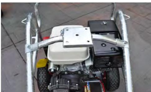
2. Fit hose reel to the mounting plate using the four sets of nuts and bolts supplied. Ensure all bolts are securely tightened and use Loctite to prevent them vibrating loose. The reel should be positioned so that it rotates fore/aft to aid fitting whip hose.
